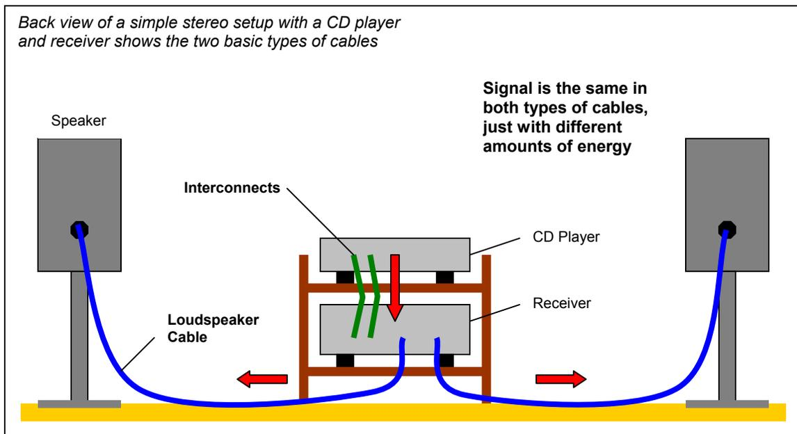
Interconnects carry a signal with very little energy. These cables only need just enough energy to convey the information from the source, for example a CD player, to the amplifier. The low energy requirement means that the signal in interconnects has very little current (usually in the range of thousandths of an amp).
